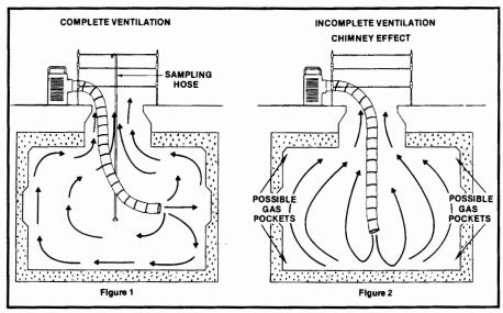
into the space while providing continuous access through the manhole without hindering worker movement or flattening the hose.
